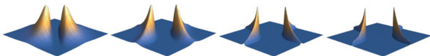
Fig. 4.8 Numerically computed optimal density \pi^\tau(r_1, r_2) in (4.89) for two electrons in one dimension and the density \rho(r) = c_0/\cosh r , r \in [-10, 10] , for different values of the regularization parameter \tau . Here c_0 is a normalization constant, and we have used the effective Coulomb interaction [7] V_{ee}(r_1, r_2) = 1.07 e^{-|r_1 - r_2|/2.39}
